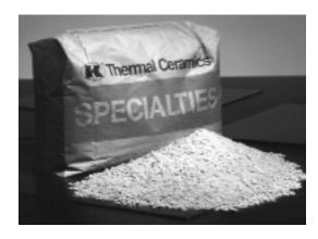
Super lightweight Kaolite castables reduce both the quantity of heat storage and heat transfer through the lining producing significant savings in furnace fuel consumption. The lower densities of these vermiculite based Kaolite castables reduce the amount of supporting furnace steel work required and provide more insulation with a thinner lining. These products can be cast, poured, or gunited.
