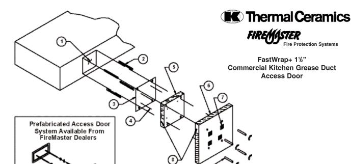
OPL Design No. GD 544 F and GD 562 F Figure 3 UL Design No. G-14 and V-19 Drawing No. FMFW1.5001-1 Door hole One layer FastWrap+ 1" overlap 2 1/4" diameter all threaded rods Speed clips 3 Access cover 16 gauge Aluminum tape at edges Insulation pins welded Spool pieces for threaded rods 5 One layer FastWrap+ 11/2" thick 10 1/4" diameter wing nuts
